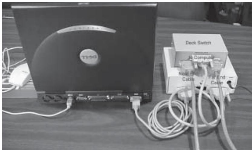
NOTE: Your starting device will work in both the NEAR END or FAR END position, regardless of which deck cable it is connected to. For example, if you normally have your start connected to the near end deck cable, it will continue to work even when you switch to the FAR END position. It is not necessary to move the start to the far end cable.
